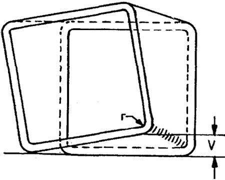
$r_{max}$  = Maximum permitted outside corner radius in mm.
