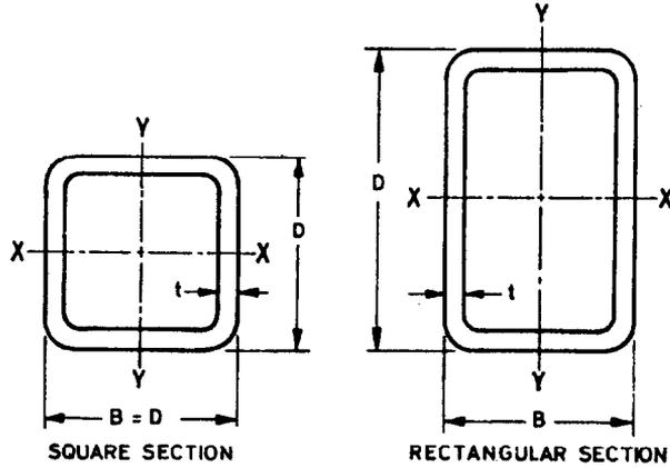
$$\text{Area of cross-section} = A = 2t [(B-4t) + (D-4t) + \frac{3}{2}\pi t] \text{ in cm}^2$$
